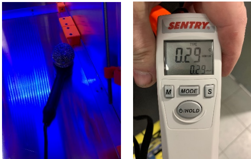
Figure 2 UVC levels inside the microphone grille
