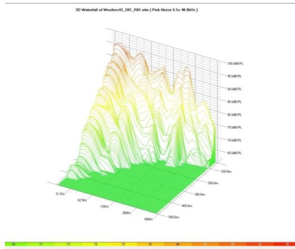
Figure 5: Waterfall plot of the room under test.
