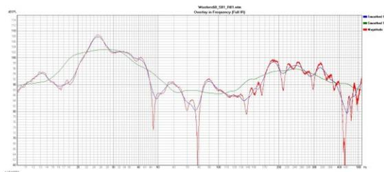
Figure 38: Overlay of the effects of smoothing on an example audio signal: red: unsmoothed; green: octave smoothed; blue: 1/6th octave smoothed
