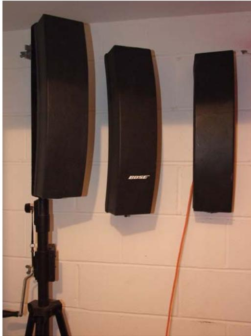
All the loudspeakers were driven from the same amplifier and the signal was transferred by moving the connector between the boxes.
